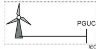
b) generating unit in a wind power plant using a wind turbine with medium rated voltage
